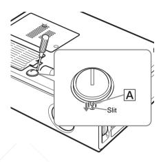
**3** When opening/closing the lens protector, turn the groove of the adjuster with a coin.
