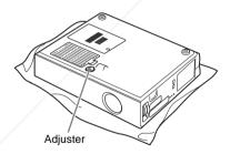
2 Slide switch A in the slit in front of the adjuster in the direction of the arrow with the small minus screwdriver.
