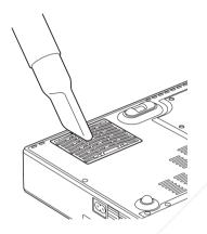
When it becomes difficult to remove the dust from the filter with a vacuum cleaner, remove the air filter and wash it.
