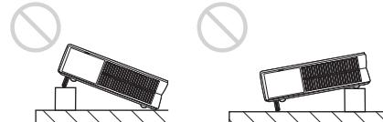
Avoid using when the unit is tilted out of the range of the adjuster setting. Such installation may cause color shading or shorten excessively the lamp life.
