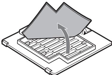
**5** Wash the air filter with a mild detergent solution and dry it in a shaded place.
