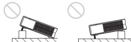
Avoid using when the unit is tilted out of the range of the adjuster setting. Such installation may cause color shading or shorten excessively the lamp life.
