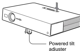
**2** Press  $\Delta$  or  $\nabla$  of the TILT key to adjust the tilt of the projector.
