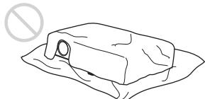
Avoid using something to cover over the ventilation holes (exhaust/intake); otherwise, the internal heat may build up.
