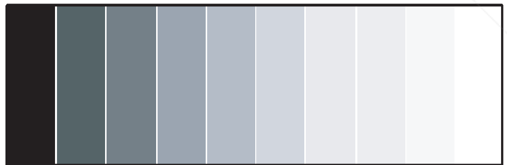
Figure 4-4. Typical Gray Bar Pattern for Adjusting Contrast
