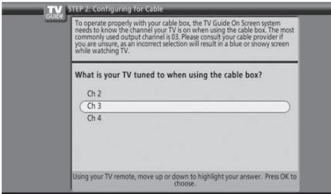
4. Highlight the channel you have to tune your TV to see cable box programming, and press OK (a screen appears reminding you to connect your G-LINK cable to your TV and cable box).
