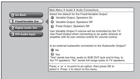
**Fixed/Variable Out** Displays a choice list that lets you turn the TV's front internal speakers on or off and set the Fixed/Variable audio output to a fixed or variable volume output level. The choices are:
