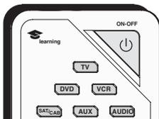
With the *Auto Tuning* feature, you can set up the TV to tune to the channel or input you want to watch by pressing that device's button. *Auto Tuning* for the *TV* button cannot be set.
