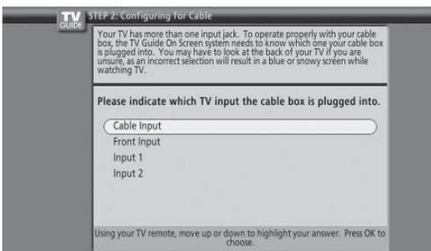
3. Highlight the input where you connected your cable box to the TV, and press OK.
