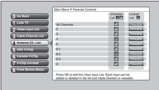
Use the *Locked List* to block a channel in your channel list if you don't want children to view the channel, for example. Selecting *Blocked* in the *Locked List* to block a channel. In the example to the left, channel 8-2 is removed from the *Antenna Ch. List*. When the TV is locked, access the channel directly by using the number buttons on the remote control then enter your valid password to view the channel.
