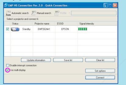
Select the "Use multi-display" check box, and click "Display properties". The "Screen properties" screen is displayed.
