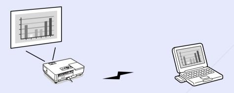
Quick Connection Mode uses an ad hoc connection (a connection among computers with a common ESSID) to connect. You can connect to a computer equipped with either of the following.
