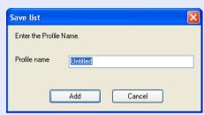
After entering the profile name and selecting the save destination, click the "Add" button because the following screens are displayed when a profile has already been created.
