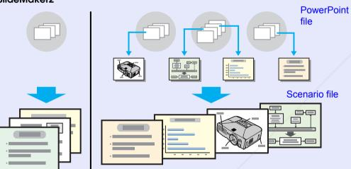
Transfer the created scenarios to store them on a USB storage device or CompactFlash card connected to the computer. Then, connect the USB storage device or CompactFlash card to the projector so that you can use the projector's PC Free function to project the scenario.
