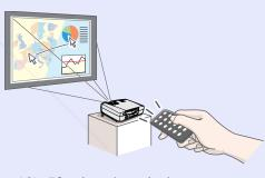
(see "Wireless Mouse Function" on ( p.19). If using the wireless mouse function, you can use the remote control to scroll back and forth through pages when projecting a PowerPoint presentation.
