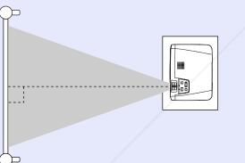
If it is not possible to set up the projector so that it is perpendicular to the screen, it can be set up at a slight vertical angle instead. You can extend or retract the front adjustable feet to adjust the upward projection angle
