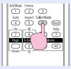
Each time you press the button, the color mode name is displayed on the screen and the color mode changes.
