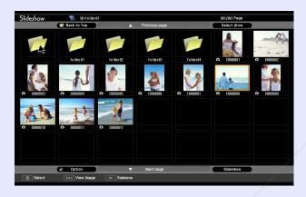
When the projector is connected to multiple storage devices, the following kind of drive selection screen is displayed containing icons that indicate the type of storage. In this case, press the [5] button, and after selecting the drive for the content you want to display, press the [Enter] button.
