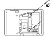
Insert the supplied screwdriver of the replacement lamp into the lamp cover opening switch, then remove the lamp cover.
