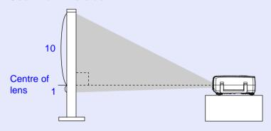
If it is not possible to set up the projector so that it is perpendicular to the screen, it can be set up at a slight vertical angle instead. You can adjust the upward projection angle of the projector to a maximum of 12° and the downward projection angle to a maximum of 4° by extending and retracting the front adjustable foot and rear adjustable feet.
