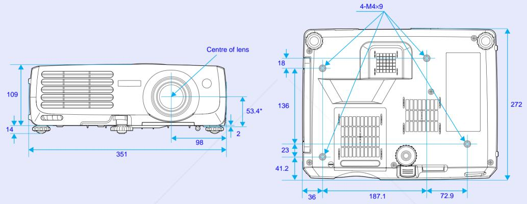
\*Distance from center of lens to suspension bracket fixing point
