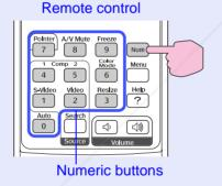
While holding down the [Num] button, press the numeric keypad buttons to enter the password. If the password is entered correctly, projection will then start.
