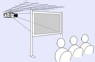
\* A special method of installation is required for suspending the projector from the ceiling. Please contact your supplier if you would like to use this installation method. The optional ceiling mount is required when installing the projector on the ceiling. • p.93
