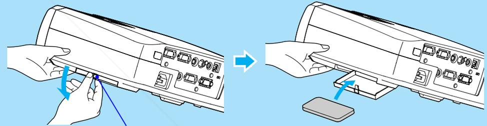
Hook a finger into the middle of the remote control holder and pull it downwards.
