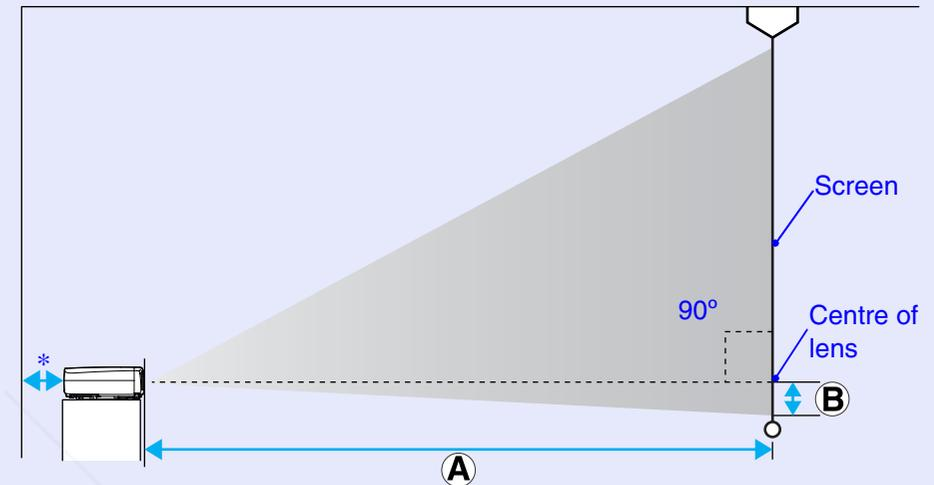
\* When installing against a wall, leave a space of about 20 cm (7.9 in.) between the projector and the wall.
