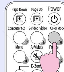
The current setting appears in the top-right corner of the screen each time the colour mode is changed.
