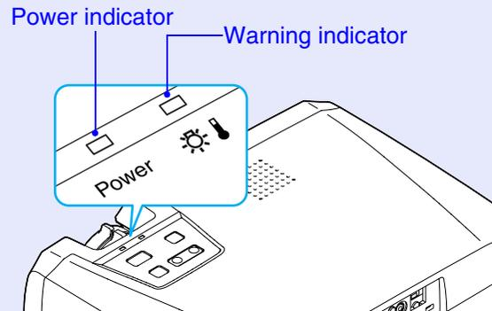
The following tables show what the indicators mean and how to remedy problems that they indicate. If both indicators are off, check that the power cable is connected correctly and that power is being supplied normally.
