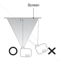
If the projector is placed at an angle to the screen, then the projected image will be distorted.
