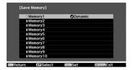
Select the memory name to register the adjustments to from Memory1 to 10, and press [Enter] or [Enter].
