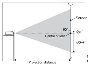
This is the height from the centre of the lens to the bottom of the projection images. It can be changed by the vertical lens shift setting.
