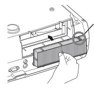
Install with the groove faced to the right.
