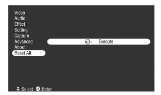
Select Reset All and press the Enter button on the control panel or remote control to display the confirmation screen. Select Yes to reset all the default settings or No to cancel.
