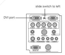
2. Using the tip of a pen or a small screwdriver, slide the DVI/VGA interface switch to the left. (If you need to use the projector's VGA port again, be sure to slide the switch back to the right.)
