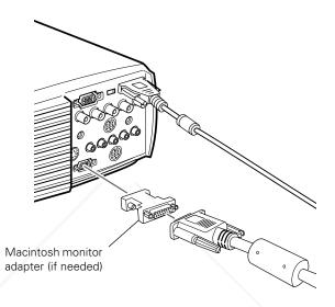
6. Tighten the screws on the connectors.
