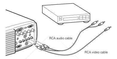
2. If you'll be using audio, connect the RCA audio cable to the left and right Audio ports of the projector (insert the white plug into the L port and the red plug into the R port). Connect the plugs at the other end of the cable to the audio output ports of the video source.
