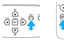
2 Select "Lamp Hours Reset" from the "Reset" menu, using the [▲][▼][←] buttons.
