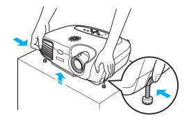
• The height can be adjusted by turning the base of the front feet on either side.
