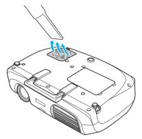
• If the air filter is difficult to clean or if it is broken, it should be replaced. Contact your dealer for a new air filter.
