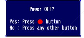
The confirmation screen disappears if anything other than the [Power] button is pressed, or if nothing is pressed for 7 seconds.
