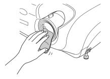
As the lens can be easily damaged, do not rub the lens with harsh materials or subject the lens to shocks.
