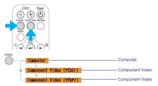
The input source switches between Computer and Component video whenever the [Computer] button is pressed, as shown above.
