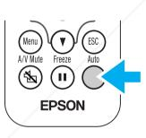
If you press the [Auto] button during E-Zoom or Freeze operation, or when a configuration menu is being displayed, the display will be halted and auto setup will take place.
