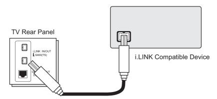
1) Connect the i.LINK cable from the back of the TV to the back of the i.LINK compatible device.
