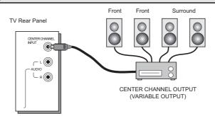
1) Connect the Pin cable from the TV's CENTER CHANNEL INPUT terminal to the surround amplifier's CENTER CHANNEL OUTPUT terminal.
