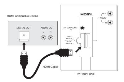
1) Connect the HDMI Cable from the DIGITAL OUT on the back of your DTV or HDMI device, to the DIGITAL-IN on the back of your television.
