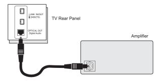
1) Connect the optical cable from the back of the TV to the back of the amplifier.
