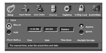
Figure 3. Clock menu. Setting the clock manually.
