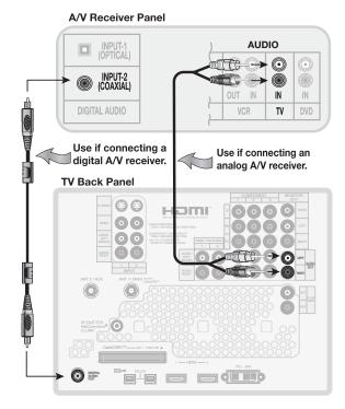
Figure 11. Connecting audio from the TV to an A/V receiver
