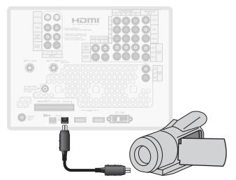
You can connect an IEEE 1394 camcorder with an IEEE 1394 cable or with analog audio/video cables. In either case, test using the TV's remote control to operate the camcorder over the IEEE 1394 cable.
