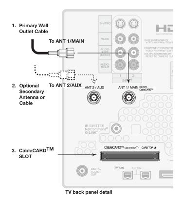
Figure 3. Wall Outlet Cable
