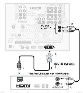
Figure 3. Connecting a personal computer with an HDMI monitor output
