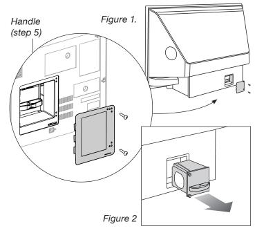
d. Carefully push in the cartridge until it is fully seated. If the cartridge does not slide in smoothly, gently wiggle the handle from side to side while pushing in.
