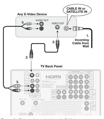
Figure 2. Connecting a device with S-Video
