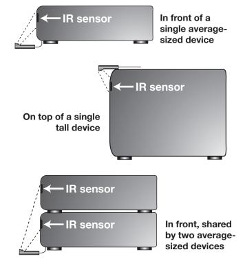
Figure 15. IR emitters so the signal can be "seen" by the IR sensor on each device.
