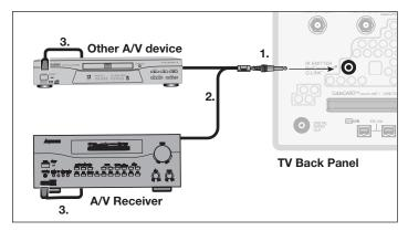
Figure 14. Connecting IR Emitter NetCommand
