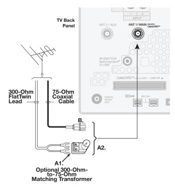
Figure 4. Connecting a Single Antenna
