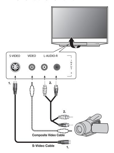
Figure 13. Analog connections for a camcorder
