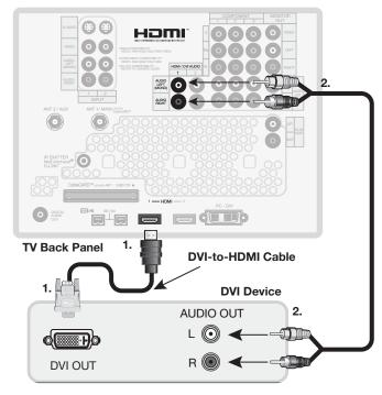
Figure 9. Connecting a DVI device
