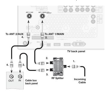
Figure 12. Connecting an older cable box
