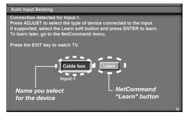
Figure 8. Highlight the Auto Input Sensing screen's Learn button and press ENTER to open the NetCommand Learn screen.
