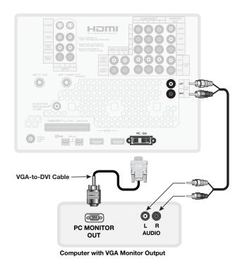
Figure 4. Connecting a computer with a VGA 15-pin monitor output.
