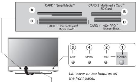
Right: **INPUT 3** and controls on front panel
