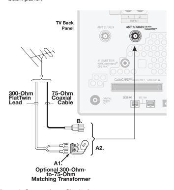
Figure 4. Connecting a Single Antenna
