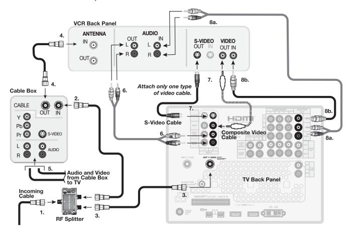
Figure 7. Connecting a VCR to a cable box
