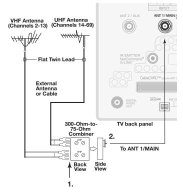
Figure 5. Connecting separate UHF and VHF Antennas
