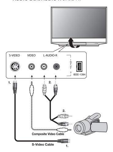
Figure 13. Analog connections for a camcorder
