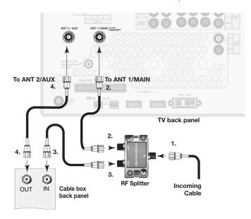
Figure 12. Connecting an older cable box
