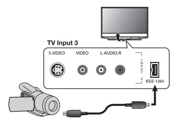
You can connect an IEEE 1394 camcorder with an IEEE 1394 cable or with analog audio/video cables. In either case, test using the TV's remote control to operate the camcorder via the IEEE 1394 cable.
