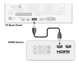
Figure 8. Connecting an HDMI device.
