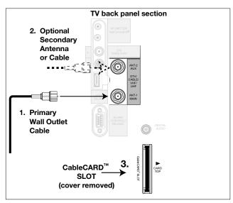
Figure 1. Wall Outlet Cable
