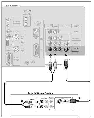
Figure 8. Connecting a Satellite Receiver with S-Video
