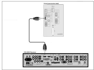
Figure 15. Connecting HDMI Device
