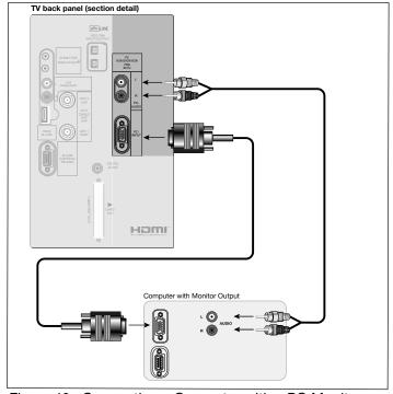
Figure 10. Connecting a Computer with a PC Monitor
