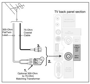
Figure 3. Connecting a Single Antenna
