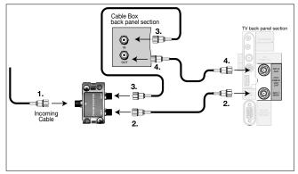
Figure 2. Connecting a Cable Box
