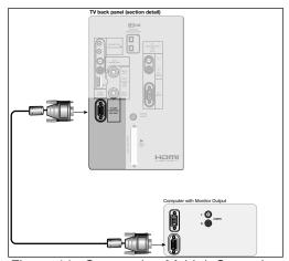
Figure 14. Connecting M-Link Control
