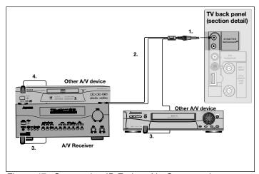
Figure 17. Connecting IR Emitter NetCommand
