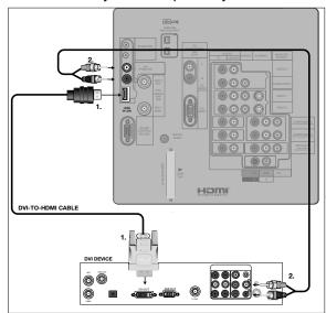
Figure 16. Connecting a DVI Device
