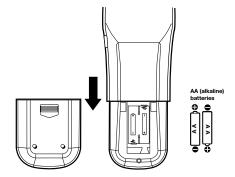
Figure 2. Operation: Installing the Batteries
