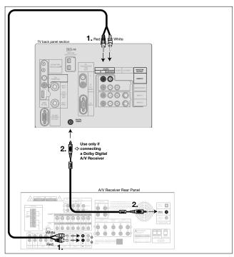
Figure 7. Connecting an A/V receiver
