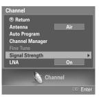
If the signal strength meter indicates that the signal is weak, physically adjust your antenna to increase the signal strength. Continue to adjust the antenna until you find the best position with the strongest signal.
