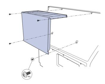
**3** Using a Phillips screwdriver, secure the shelf to the TV with the four screws that came with it. Tighten the screws.
