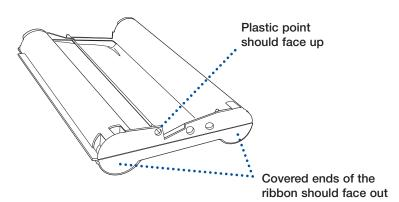
7 Carefully align the cassette and its ribbon with the slot, then gently push in the cassette until it clicks into place beneath the latch.
